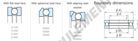
Thrust Ball Bearings - Single Direction
