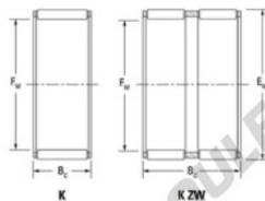
Flat/flat needle roller and cage assemblies
