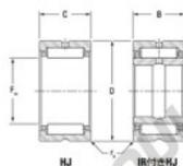
Heavy duty needle roller bearings
