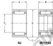
Heavy duty needle roller bearings
